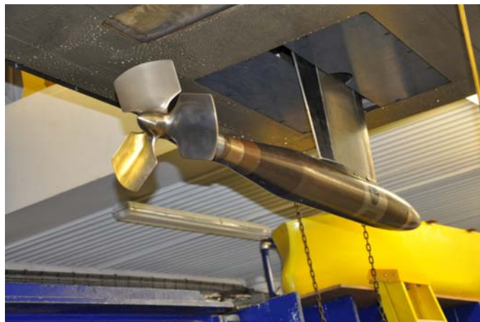
Figure 4 – Axiom propeller attached to the H33/45 K&R open water dynamometer
